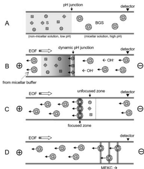
**Figure 10.** Schematic diagrams of the dynamic pH junction-sweeping model. (A) The micellar (such as SDS) BGS and the sample solution (a nonmicellar buffer) are injected into the capillary, respectively; (B) when the injection is complete, a positive polarity is applied (if a negatively charged SDS surfactant is used) to power the CE separation; (C) the neutral analytes are converted to anions and are swept by the SDS micelles; (D) separation occurs by the MEKC mode.
