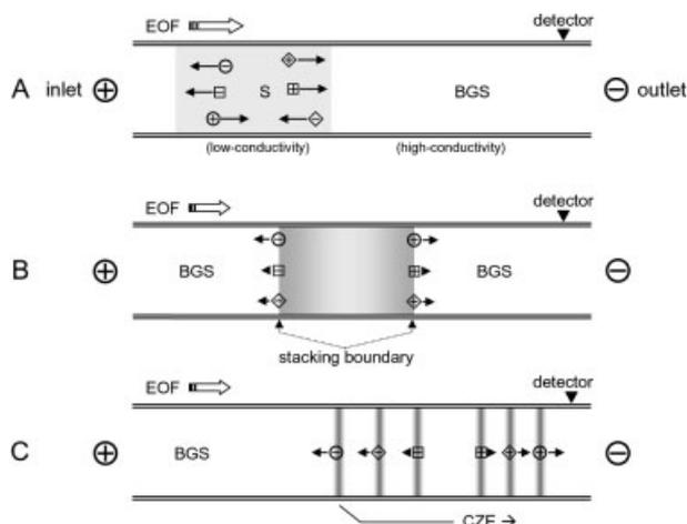
**Figure 1.** Schematic diagrams of the FASS model. (A) The capillary is conditioned with a BGS (a high conductivity buffer), the sample, prepared in a low-conductivity matrix, is then injected to a certain length, and a high positive voltage is applied; (B) focusing of the analytes occurs near the boundaries between the sample zone and the BGS because of its mobility changes; (C) stacked analytes migrate and are separated by the CZE mode.
