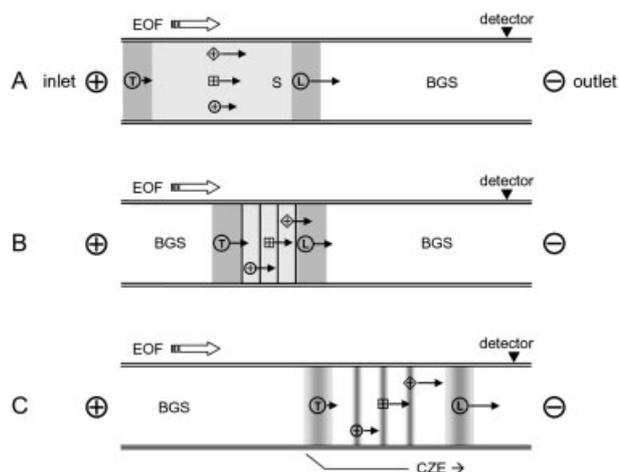
**Figure 11.** Schematic diagrams of a tr-ITP model for cations. (A) The capillary is conditioned with a BGS, the leading electrolyte, sample solution, and terminating electrolyte are then injected in turn, and a high positive voltage is applied; (B) concentration of the analytes occurs between the leading and the terminating ions during tr-ITP migration; (C) the concentrated analyte zones are separated by the CZE mode.
