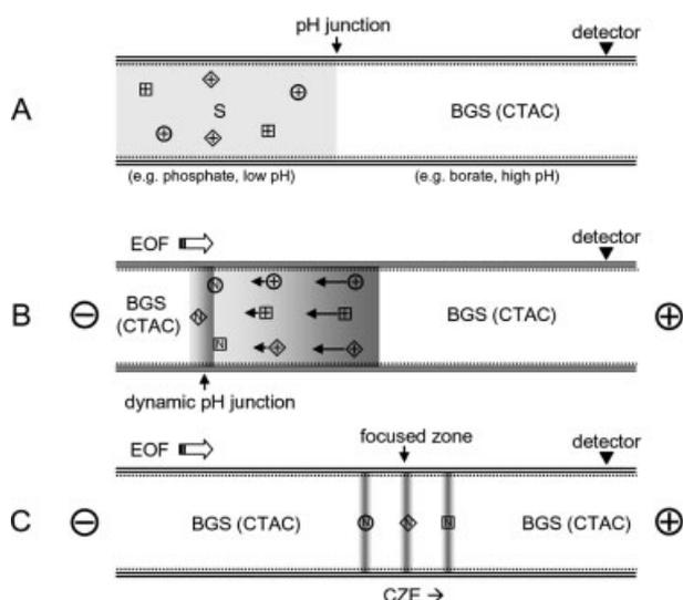
**Figure 9.** Schematic diagrams of the reversed dynamic pH junction model. (A) The capillary is filled with BGS (prepared in a higher-pH buffer containing CTAC) and sample solution (prepared in a lower-pH matrix); (B) a negative voltage is applied because of the addition of CTAC the EOF moves toward the outlet; the cationic analytes move toward the inlet and change to neutral at the rear boundary due to the change in pH; (C) separation of the analytes occurs by the CZE mode.
