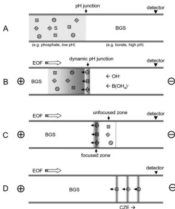
**Figure 8.** Schematic diagrams of a dynamic pH junction model. (A) The capillary is filled with a high pH-BGS and a section of sample solution (prepared in a lower-pH buffer); (B) a high positive voltage is applied, resulting in a discontinuous electrolyte zone; (C) the anionic analytes are focused on the boundary of the pH junction; (D) separation of the analytes occurs by the CZE mode.
