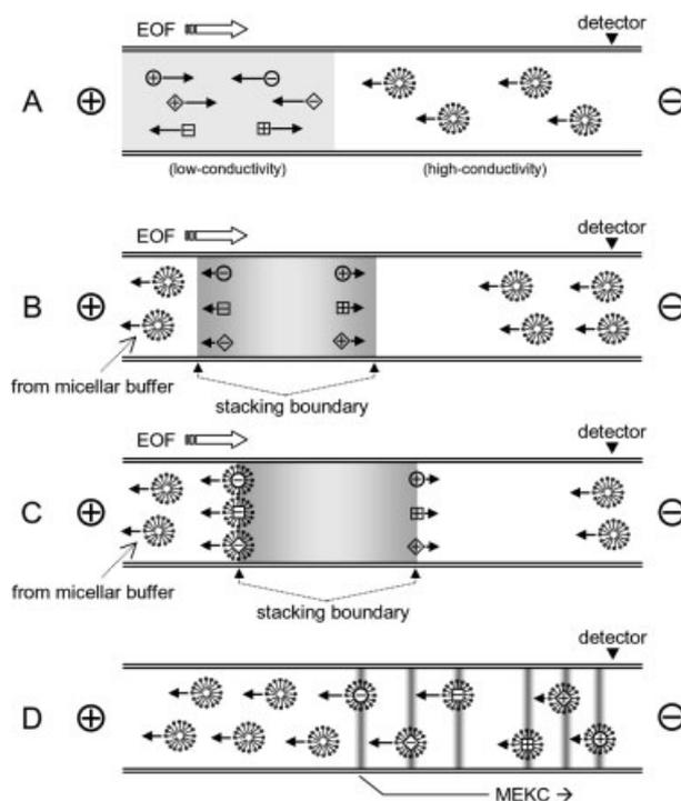
**Figure 4.** Schematic diagrams of a normal-stacking MEKC model. (A) The sample is dissolved in a low-conductivity buffer, BGS, consisting of SDS to form the micelles; after the background and sample solution are injected, respectively, a positive voltage is applied; (B) the SDS micelles from the inlet enter the sample zone and then permit the analytes to migrate and become stacked; (C) then the SDS-analytes are separated by the MEKC mode.
