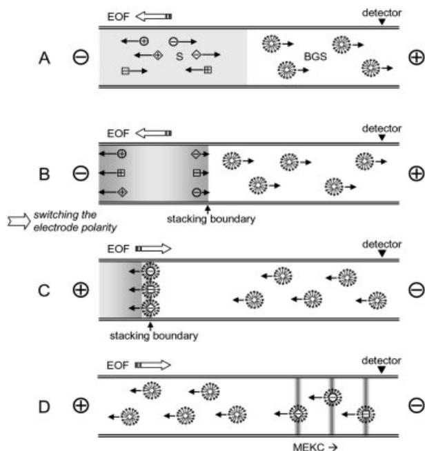
**Figure 5.** Schematic diagrams of a reversed-stacking MEKC model. (A) The sample and BGS are prepared as described in Fig. 4A but a negative polarity is applied; (B) the EOF moves toward the inlet, the anionic analytes move toward the outlet and stack at one side of the boundary; (C) the electrophoretic current reaches approximately 95–99% of its original value, the polarity is quickly returned to positive, reversing the EOF; (D) then the SDS-analytes are separated by the MEKC mode.
